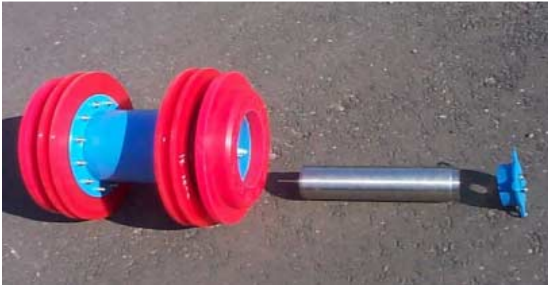
Figure 1 – Bidi Pig and SAAM Unit
