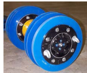
Fig. 3 A typical SAAM carrier pig
