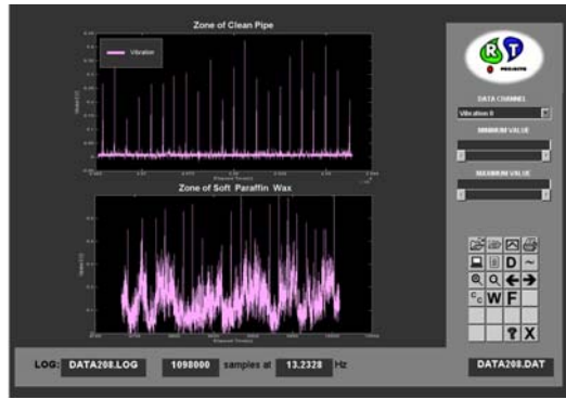
Fig. 8 Pig Behaviour in Soft Wax
