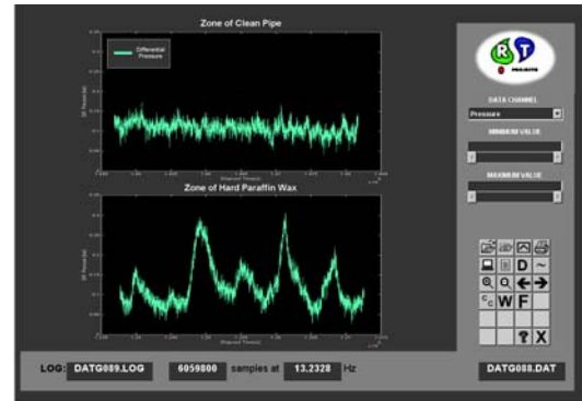
Fig. 9 Pig Behaviour in Hard Wax
